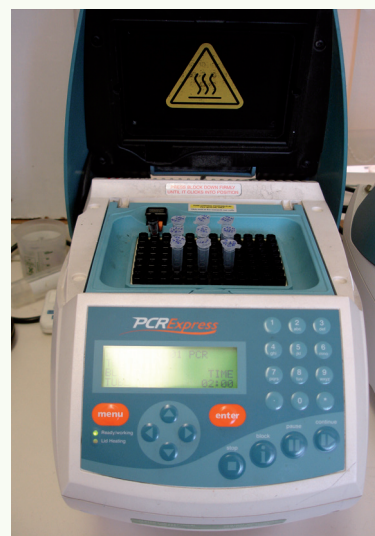
Box figure 4.2 – A typical thermocycler, used to carry out PCR amplification.
