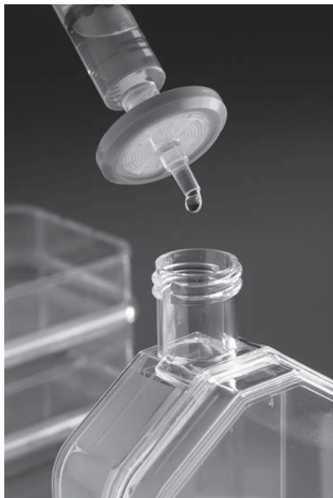
Fig. 21.9 Using a sterile filter. In this example, the Millipore® filter is attached to a plastic syringe, used to take up and expel the liquid.
