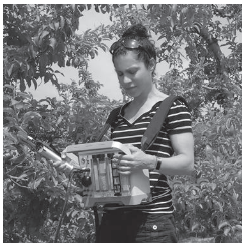
Fig. 71.2 A portable infrared gas analyser, used to measure photosynthetic \text{CO}_2 uptake (leaf cuvette/probe shown in left hand, with analysis unit and user interface below).
