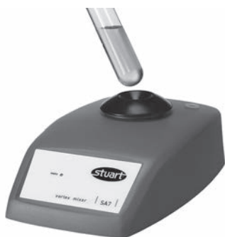
Fig. 21.7 Example of a vortex mixer. The test tube is gently engaged with the orbitally vibrating rubber holder to impart a spinning motion to the liquid within. In some models, the holder can be replaced by an insert for operation with multiple sample vials, e.g. Eppendorf tubes.
