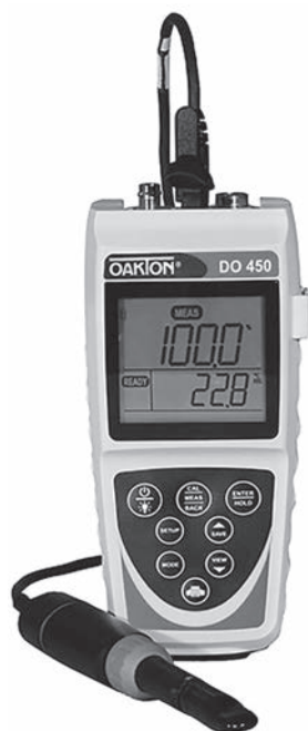
Fig. 70.5 A typical optical DO instrument for use in the field, the Oakton DO 450. This instrument has a resolution of 0.1 \text{ mg L}^{-1} (ppm w/v) and an accuracy within 2% of full saturation, with inbuilt compensation for temperature, pressure and salinity. It can store several hundred manual or timed readings which can then be downloaded later.
