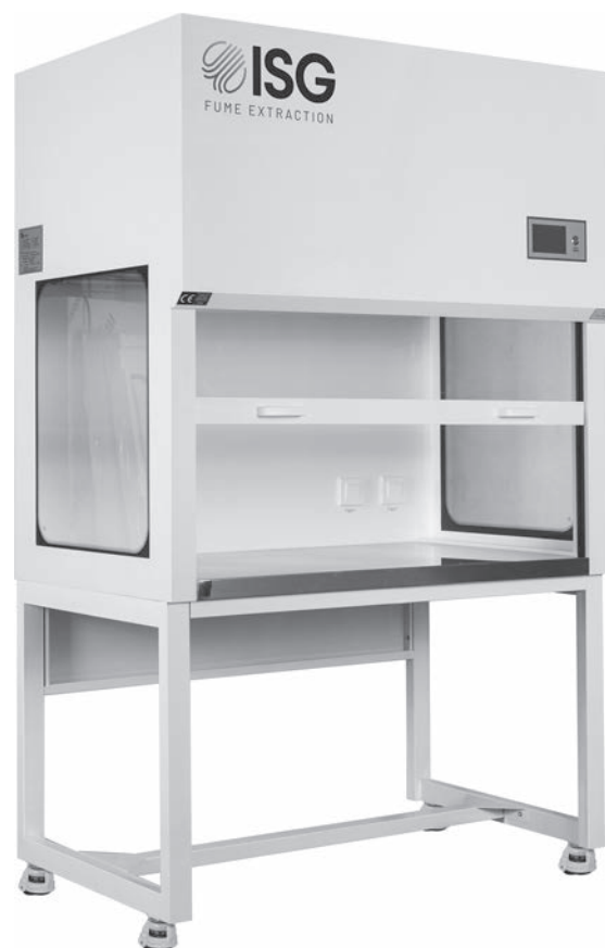
Fig. 47.4 A laminar flow cabinet. Air is drawn in and through a HEPA filter in either the back or the top, exiting the front through the opening created by the moveable glass door. When in use, raise door only enough to enable you to work on the workbench.
