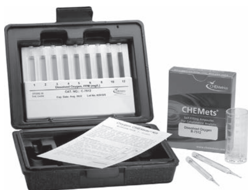
Fig. 70.3 Example of a CHEMetrics colorimetric Dissolved Oxygen test kit. Color-forming reagent is sealed under vacuum in self-filling glass ampoules. Water sample is drawn into the ampoule and mixed with the reagent. The color intensity from the reaction is compared with the color standards provided.
