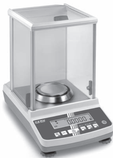
Fig. 21.2 Example of a self-taring electronic balance. Note the shield to help stabilise readings by reducing air flow around the machine.
